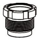
**NOTE:** Only the 45:1 pumps have shims placed on top of the female gland.
